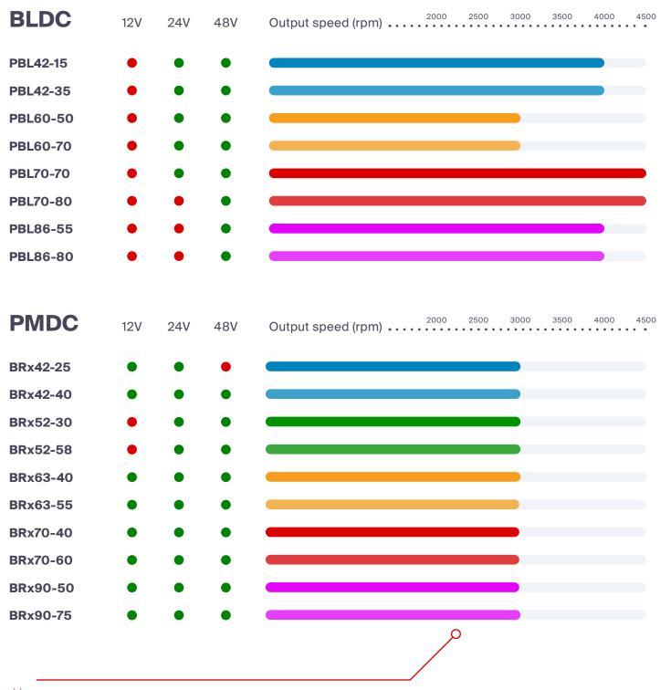
Motors in the modular range are currently only available in the speed shown above. Our standard motors can be customised to produce an output speed of 1500 - 4500 rpm.
